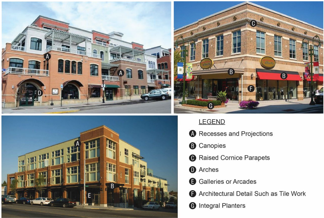
FIGURE 5.1.3.D.10.A: MIXED-USE BUILDING ENTRANCES
