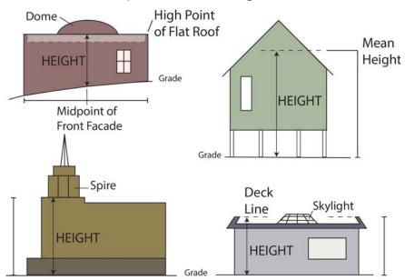
This is an example image from a rules of measurement section showing how maximum building height is determined for different kinds of roofs.
