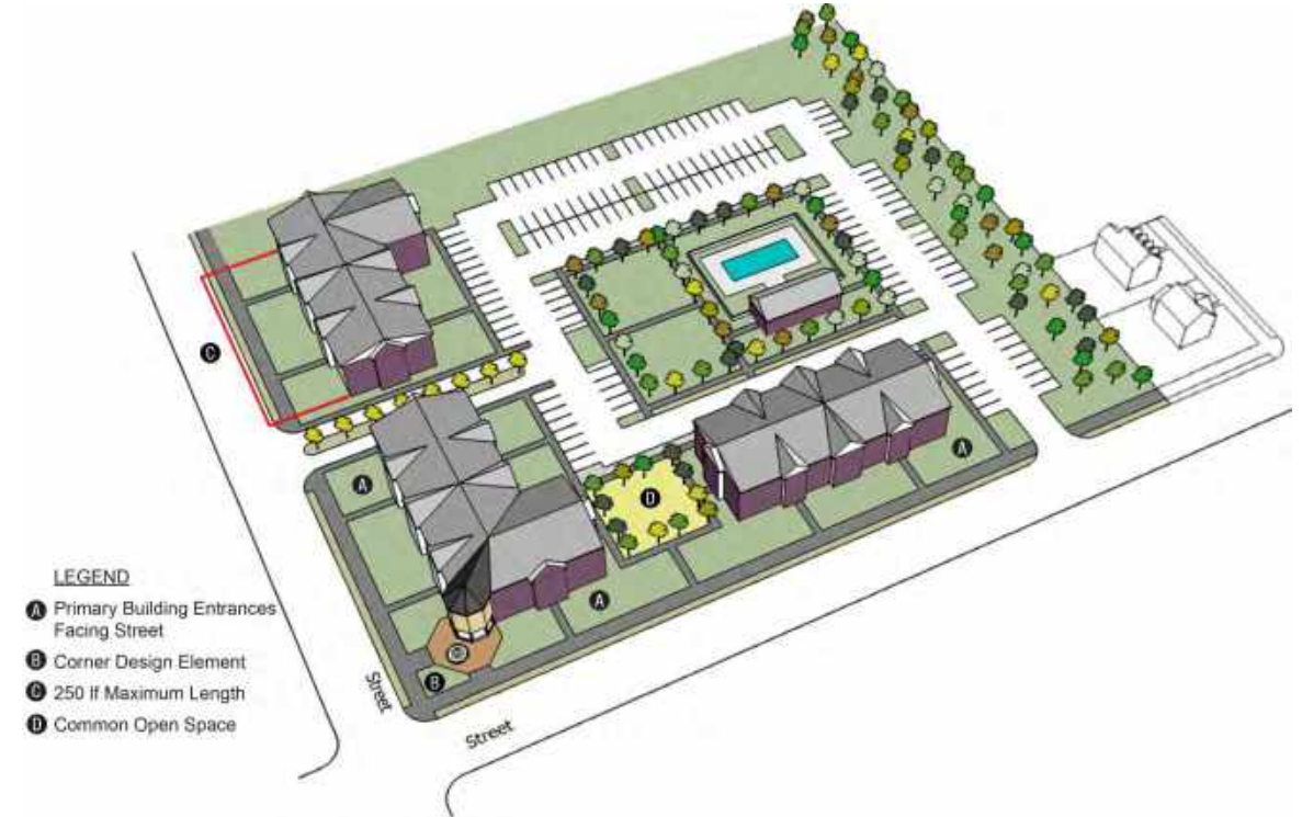
FIGURE 5.1.1.D.4: MULTI-FAMILY BUILDING ORIENTATION
