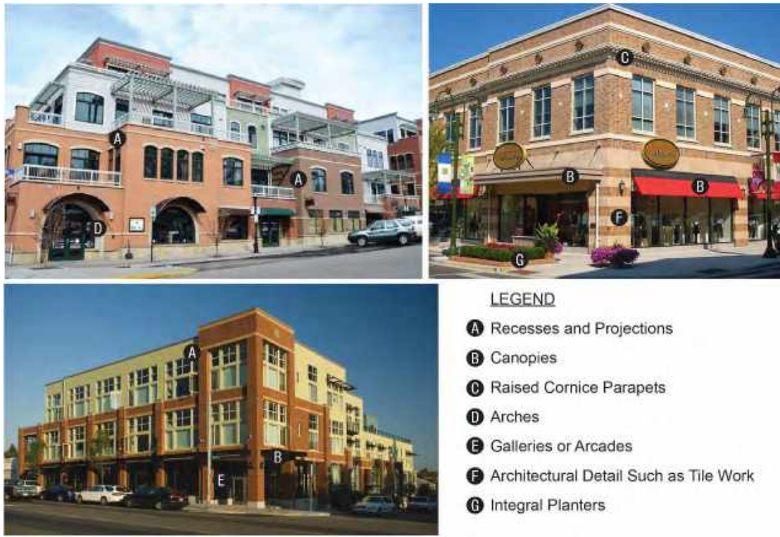
FIGURE 5.1.3.D.10.A: MIXED-USE BUILDING ENTRANCES
